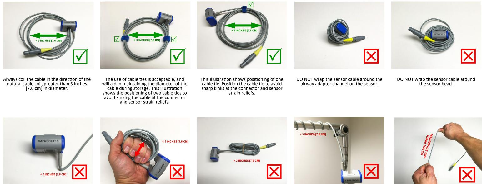
DO NOT kink the sensor cable, or bend the sensor cable less than 3 inches [7.6 cm] in diameter.
